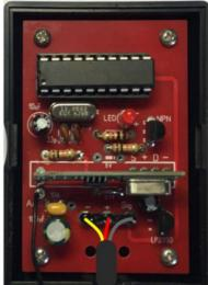
The new board is designed for 433 modules 5 volts or 3 volts voltage. For 5 volt modules, the bridge must be "5 V" above the module must be soldered.
