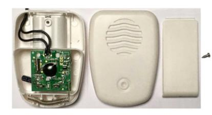
Close the housing, hook in at the top, antenna and press together. Screw on the screw.
